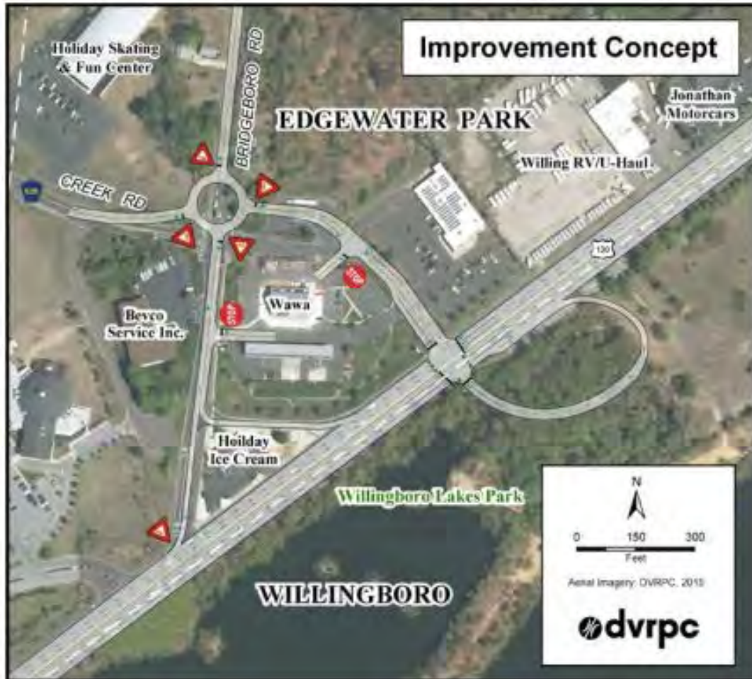
Figure 7: Proposed Improvement Concept for the US 130-Bridgeboro Road Corridor
