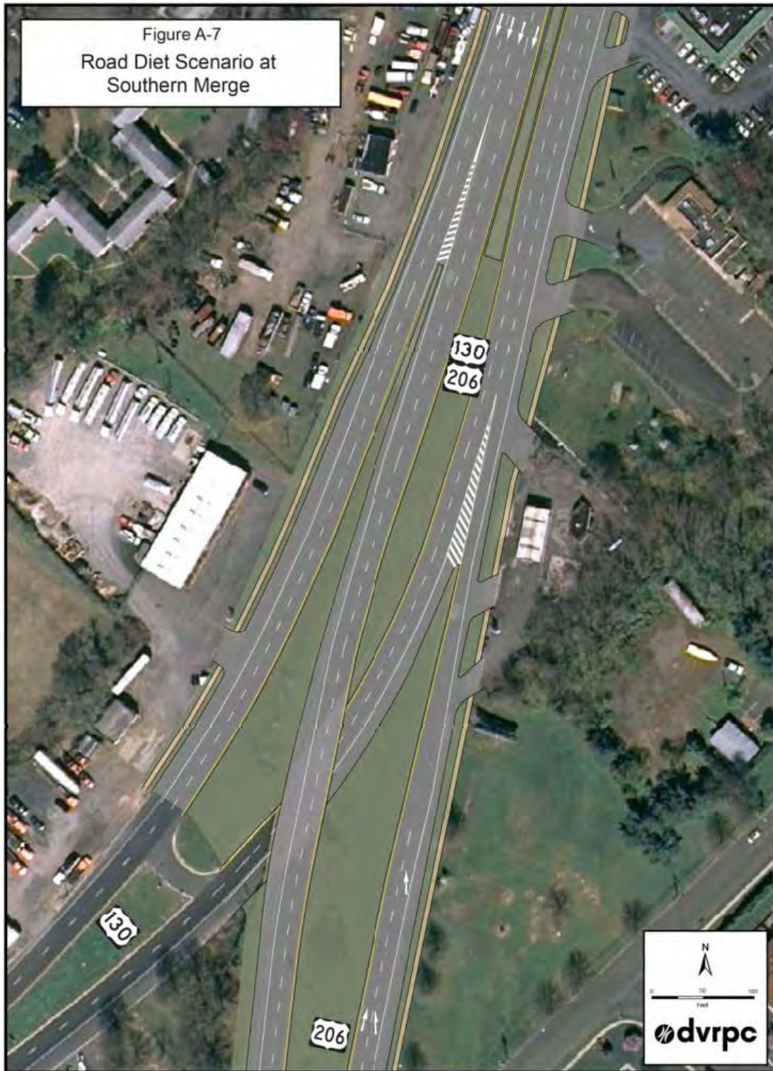
Figure 6: Proposed Improvements for US 130/US 206 Merge Area
